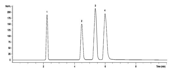
Column: Luna® 5 μm C8 100 Å LC Column 150 x 4.6 mm
